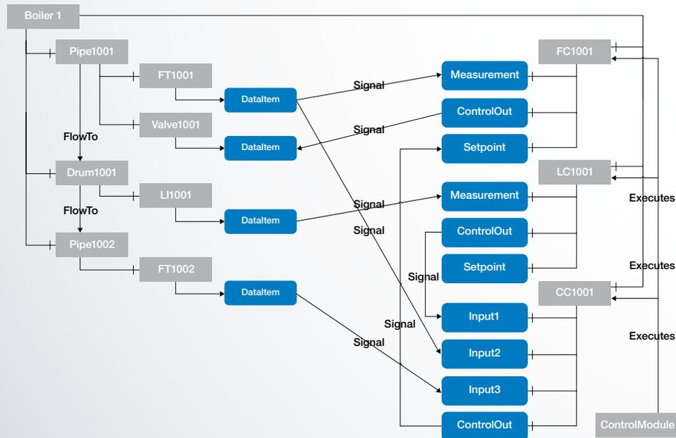
UA modeling of a boiler as an example
